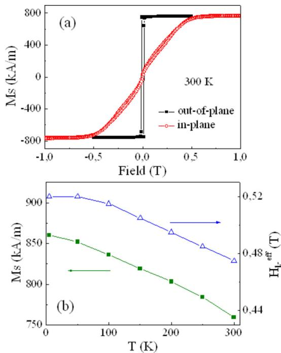
FIG. 2. (Color online) (a) Saturation magnetization vs applied field measured for a [Co(0.4 nm)/Pt(0.7 nm)]  $\times$  4 film at 300 K with out-of-plane (black solid squares) and in-plane (red open circles) field orientation. (b) Saturation magnetization (green solid squares) and anisotropy field (blue open triangles) vs temperature.
