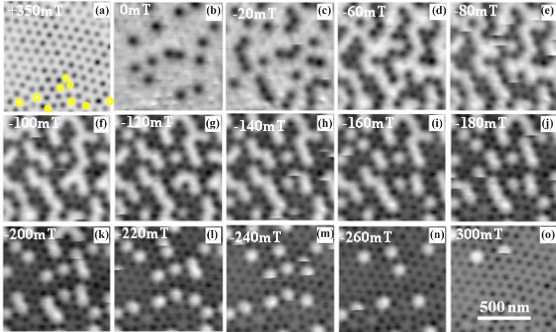
FIG. 7. (Color online)  $1 \mu\text{m} \times 1 \mu\text{m}$  MFM images obtained successively after saturation at  $+350 \text{ mT}$  (a), under  $0 \text{ mT}$  to  $-300 \text{ mT}$  (b)–(o). Since the magnetization is saturated at  $-350 \text{ mT}$ , (a) corresponds to an average topography signal that is used to correct all the other MFM images. Yellow hexagons in (a) mark lattice stacking faults.
