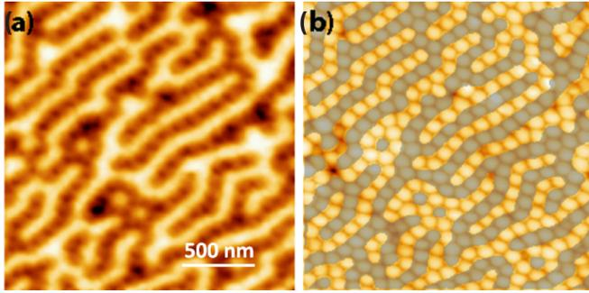
FIG. 12. (Color online) (a) MFM image of a  $2\ \mu\text{m} \times 2\ \mu\text{m}$  array of bumps sample surface. (b) Corresponding  $2\ \mu\text{m} \times 2\ \mu\text{m}$  AFM image with the MFM pattern superimposed on it.
