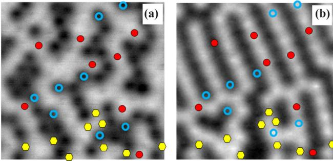
FIG. 9. (Color online)  $1\ \mu\text{m} \times 1\ \mu\text{m}$  MFM images obtained close to half reversal ( $-60\ \text{mT}$ ) after negative field saturation (a) and at remanence after demagnetization (b). The solid red disks correspond to hard switchers, open blue disks to easy switchers, and yellow hexagons to topological defects.
