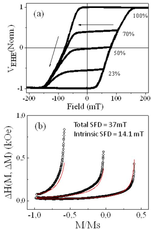
FIG. 6. (Color online) (a) EHE measurement of out-of-plane major and minor loops for Co/Pt nanobump array with  $p = 100$  nm. The percentage values correspond to the ratio of switched nanobumps during each loop. (b)  $\Delta H(M, \Delta M)$  data (open circles) obtained from the partial reversal curves in (a) and compared with the fit (red solid line) of the  $\Delta H(M, \Delta M)$  model. The quality of the fit is attested by the correlation coefficient  $R^2 = 0.9689$ .
